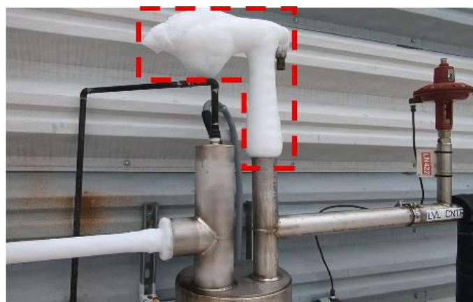
Figure 1. Ice ball formation on the LN 2 phase separator (highlighted in dashed red box), leading to increased boil-off through pressure regulator valve impediment.
